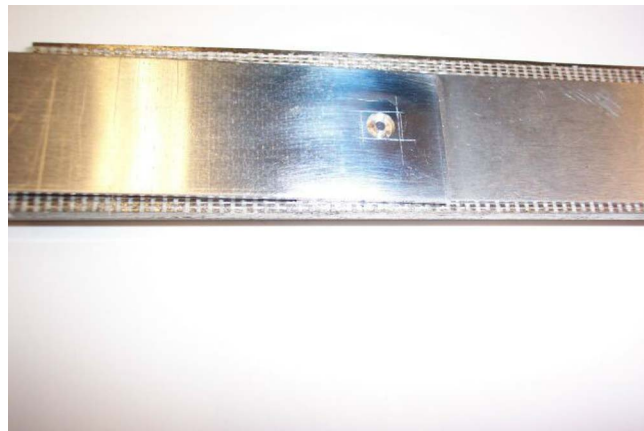
Fig. 8 Bottom surface of spot-weld coupon after the ring-core cutting
